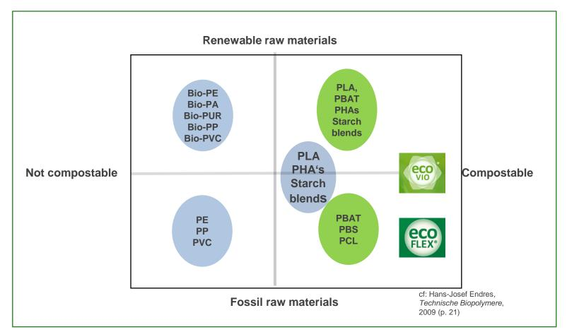
Biodegradability is based on molecular structure; therefore, both fossil-based and biobased polymers can biodegrade by action of naturally occurring microbes in organics recovery processes.
